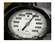
NewRider's 3000 psi, high pressure airless pump atomizes paint more efficiently than other lower pressure stripers. This allows for nearly 30% more coverage per gallon of paint at 450 linear feet per gallon, making NewRider stripers one of the most efficient ride-on athletic stripers on the market.
