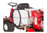
The large 50-gallon onboard paint tank allows you to spend more time painting and less time refilling your paint supply. A single tank provides enough coverage to paint up to 9 regulation soccer fields or 5 football fields.
