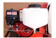
The onboard 2.5-gallon purge tank lets you clean your spray gun and hose right in the field and the inline filter keeps the system running without frustrating clogs.
