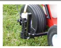
The FieldLiner 3 Deluxe's removable inline spray gun produces 2" to 6" wide lines and the 5' extension hose can be used to paint stencils and hard to reach areas. There is a cleanable strainer within the spray gun for easy maintenance.
