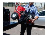
While made using durable components, the EcoLiner LT is engineered with weight savings in mind and as an alternative to more expensive self-propelled machines. Its light weight allows for much easier pushing over athletic fields and easy one-person loading and unloading when striping multiple locations.
