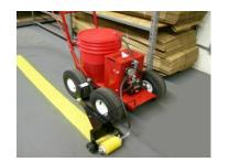
With lines up to 5 times thicker than aerosol paint and without overspray, the RollMaster 5000 can stripe even in food warehouse where gas machines cannot be used. It can also paint between cars without fear of overspray. The paint rollers ensure a crisp, clean line of paint with high visibility and durability.
