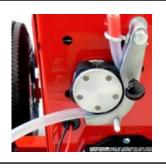
The RollMaster's peristaltic roller pump never touches your paint meaning no clogs and produces no fumes so you can use this versatile machine anywhere, including food warehouses.
